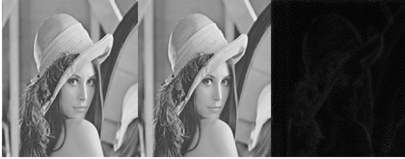
Original and watermarked images with method 3, for \alpha = 1.5 , PSNR=35.63 dB; Difference image, amplified 8 times.
