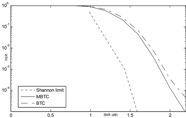
Figure 8. FER performance for 3/5 rate Turbo Coded,  $H=[11\ 1\ 12]$  and Multi Binary Turbo Coded,  $H=[11\ 11\ 1\ 12]$  transmission over AWGN channel and the Shannon limit are plotted as functions of SNR.
