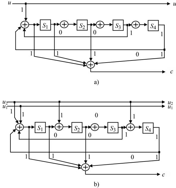
Figure 1. a) The constituent RSC encoder for TC; b) The constituent RSC encoder for MBTC. Both encoders have feedback= $(23)_8=(10011)_2$  and redundancy= $(35)_8=(11101)_2$  polynomials.
