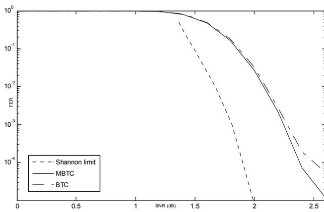
Figure 6. FER performance for 2/3 rate Turbo Coded,  $H=[11\ 1\ 12]$  and Multi Binary Turbo Coded,  $H=[11\ 11\ 1\ 12]$  transmission over AWGN channel is plotted as function of SNR. There is also plotted the Shannon limit.
