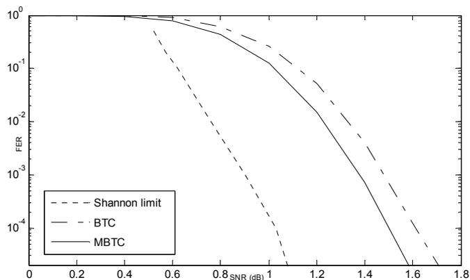
Figure 4. Frame Error Rate (FER) performance for 1/2 rate Turbo Coded,  $H=[11\ 1\ 12]$  and Multi Binary Turbo Coded,  $H=[11\ 11\ 1\ 12]$  transmission over AWGN channel and the Shannon limit are plotted as functions of SNR.
