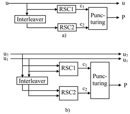
Figure 2. a) Turbo code encoder with 1/2 RSC encoders; b) Multi binary turbo code with 2/3 RSC encoders.
