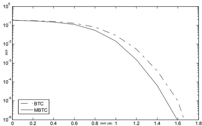
Figure 3. Bit Error Rate (BER) performance for 1/2 rate Turbo Coded,  $H=[11\ 1\ 12]$  and Multi Binary Turbo Coded,  $H=[11\ 11\ 1\ 12]$  transmission over AWGN channel, is plotted as function of SNR.
