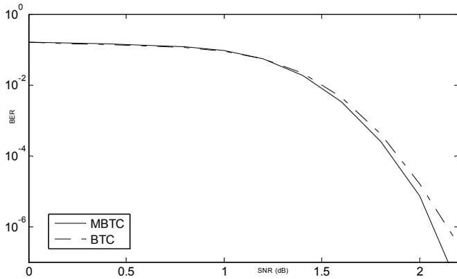
Figure 7. BER performance for 3/5 rate Turbo Coded,  $H=[11\ 1\ 12]$  and Multi Binary Turbo Coded,  $H=[11\ 11\ 1\ 12]$  transmission over AWGN channel is plotted as function of SNR.
