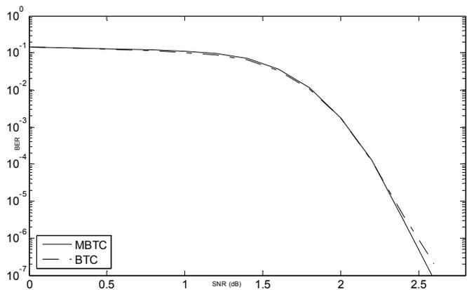
Figure 5. BER performance for 2/3 rate Turbo Coded,  $H=[11\ 1\ 12]$  and Multi Binary Turbo Coded,  $H=[11\ 11\ 1\ 12]$  transmission over AWGN channel is plotted as function of SNR
