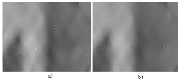
Figure 2. The proposed denoising system b) corrects some distortions introduced by the bishrink filter a).
