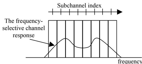
Fig. 1: The frequency-selective channel response and the relatively flat response on each subchannel
