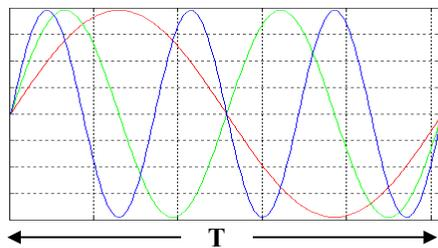
Fig. 4: The waveform of the carriers in an OFDM transmission
