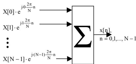
Fig.5: The multicarrier modulation using IDFT
