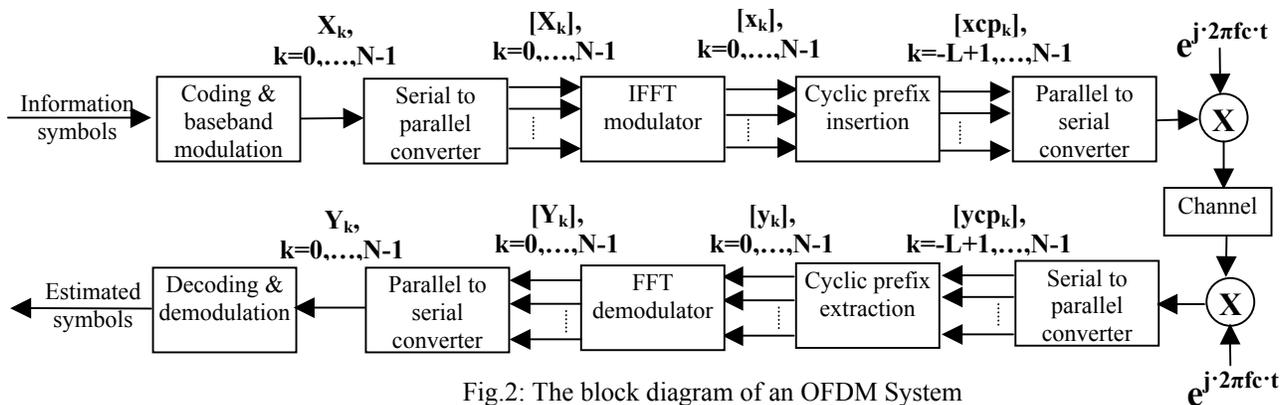
Fig.2: The block diagram of an OFDM System
