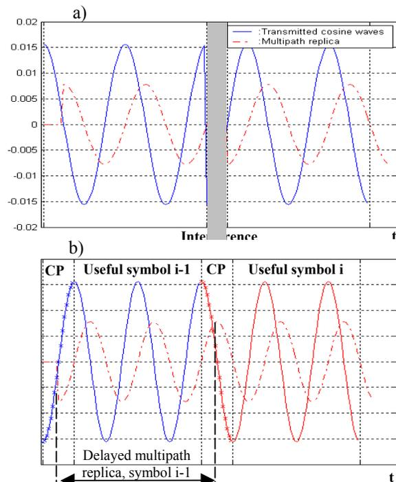
Fig. 7: IBI-two adjacent OFDM symbols interfere(a), the cyclic prefix eliminates this interference (b)
