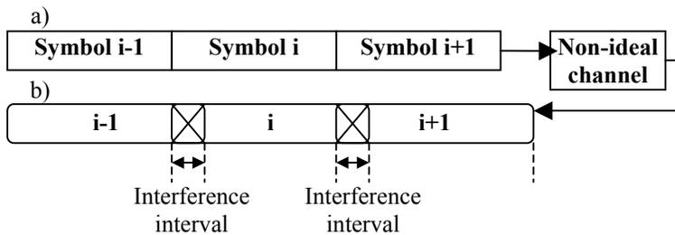
Fig.6: The transmitted symbols frame structure (a) and the received symbols are overlapping during the “interference interval”(b)
