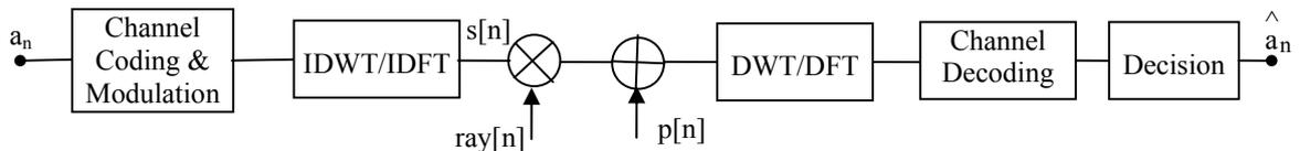
Fig.1: Transmission chain used for simulation.
