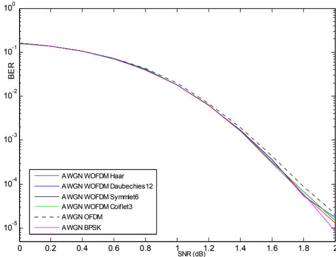
Fig.2: WOFDM versus OFDM in AWGN channels.
