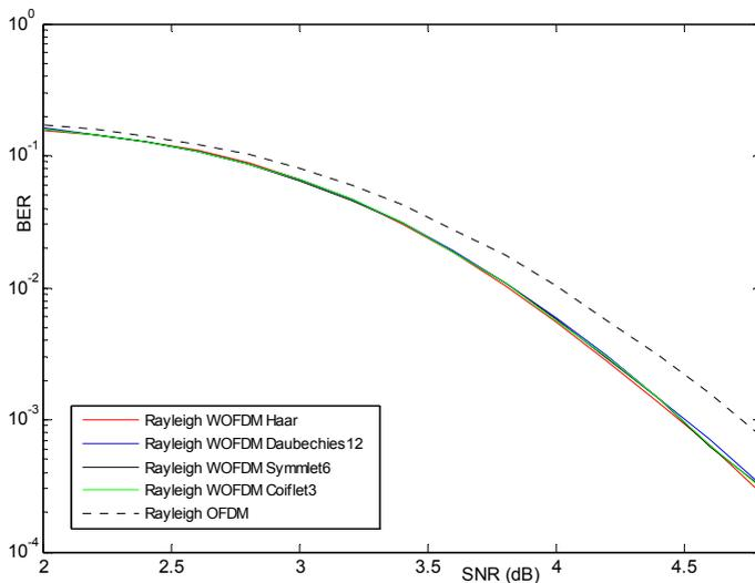
Fig.3: WOFDM versus OFDM in flat fading channels.
