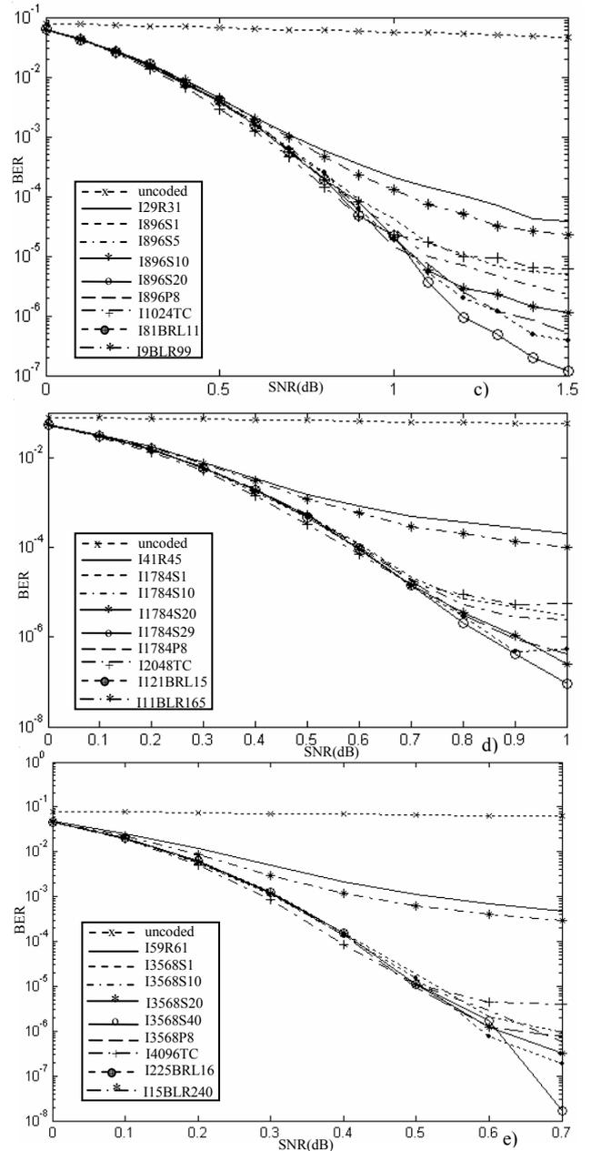
Figure 1. BER performance for the 8-state, rate 1/3, (1, 15/13), turbo code for interleavers with  $N \cong 400$  (a),  $b$ ),  $N \cong 900$  (c),  $N \cong 1800$  (d),  $N \cong 3600$  (e).
