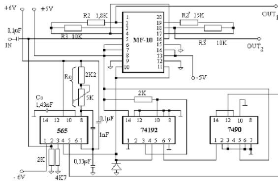
Figure 4. A tracking filter realized using the switching capacitors filter MF-10, the PLL 565 and a frequency multiplier realized with two counters. The instantaneous frequency of the input signal is detected with the PLL system. A multiple of this frequency is used to generate the clock for the switching capacitors filter.
