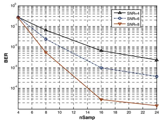
Fig. 3. The dependence of GMSK demodulation performance on the sampling rate of the EKF algorithm for different values of SNR in the case BT = 0.3.
