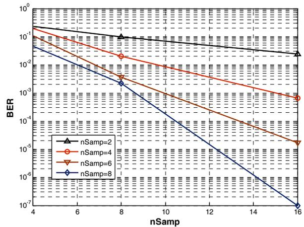
Fig. 2. The dependence of MSK demodulation performance on the sampling rate of the EKF algorithm for different values of SNR.
