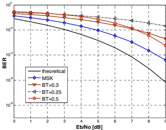
Fig. 5. The comparison of performances of MSK and GMSK signal detection by EKF for the sampling rate  $nSamp = 8$ .
