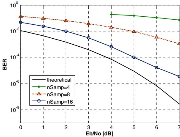
Fig. 4. The dependence of MSK demodulation performance on SNR for different values of sampling rate of EKF algorithm.
