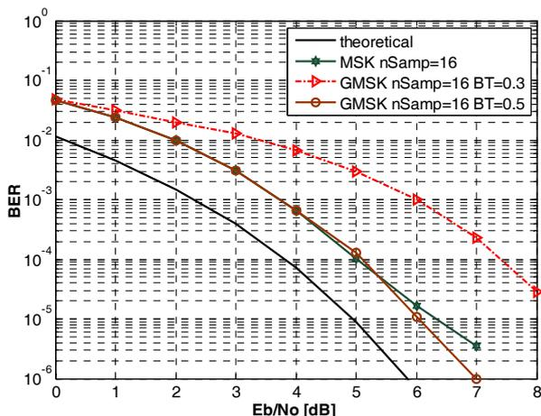
Fig. 6. The comparison of performances of MSK and GMSK signal detection by EKF for the sampling rate  $nSamp = 16$ .
