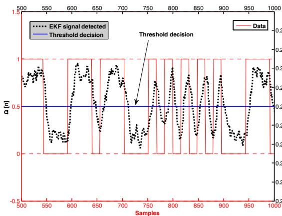
Fig. 1. MSK with SNR=8dB signal detected by EKF.
