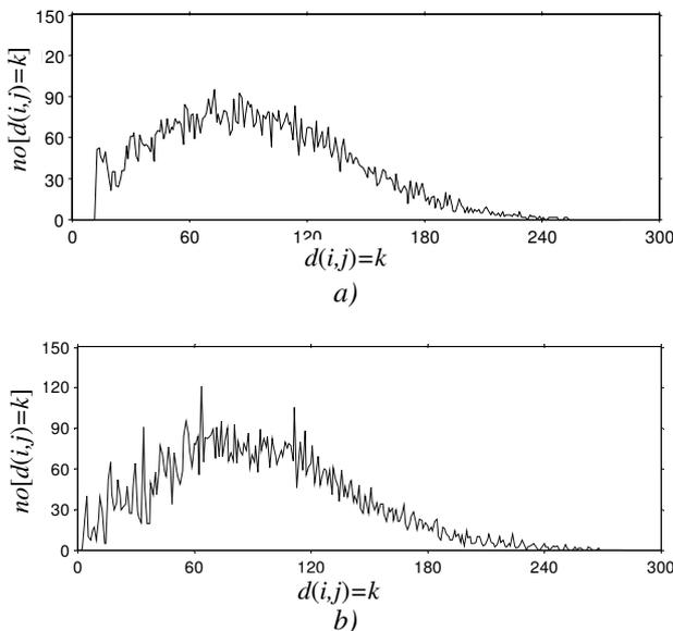
Figure 2. The DS for: a) the S-interleaver with  $S=13$  and  $N=140$ ; b) the permutation system defined by the positions sequence of the 140 sub-carrier frequencies of BS segment 0.
