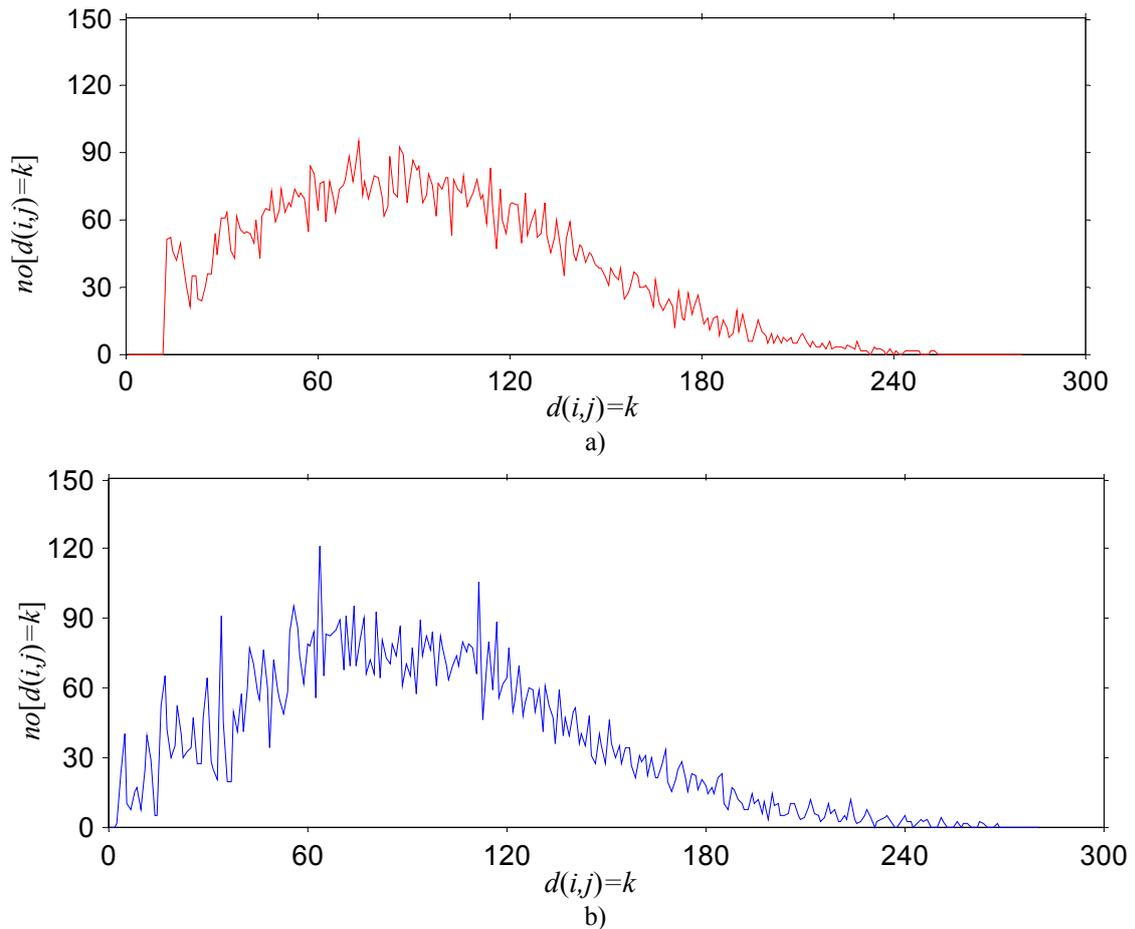
Fig. 2 The DS for: a) the S-interleaver with  $S=13$  and  $N=140$ ; b) the permutation system defined by the positions' sequence of the 140 sub-carriers' frequencies of a BS segment.
