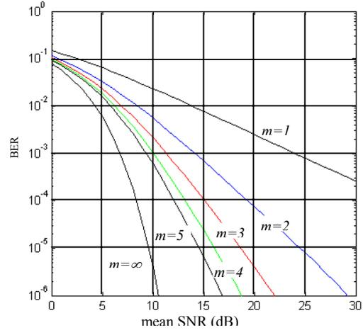
Fig. 4 The BER performances obtained through the simulation of the BPSK modulation transmission system on the Nakagami flat fading channels, with  $m=2, 3, 4$  and  $5$ .
