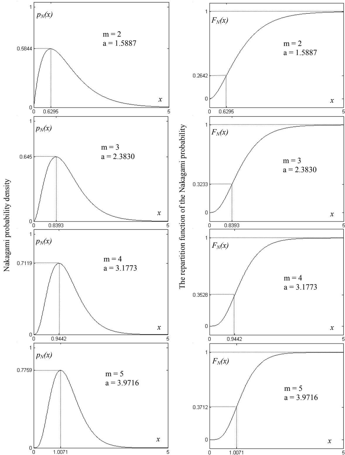
Fig. 2 The probability density and the repartition function of the probability for a random variable distributed Nakagami, with the mean  $1.2589=10^{0.1}$ .
