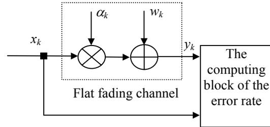
Fig. 1 Model for the simulation and for the study of the BER performances of the flat fading channels.
