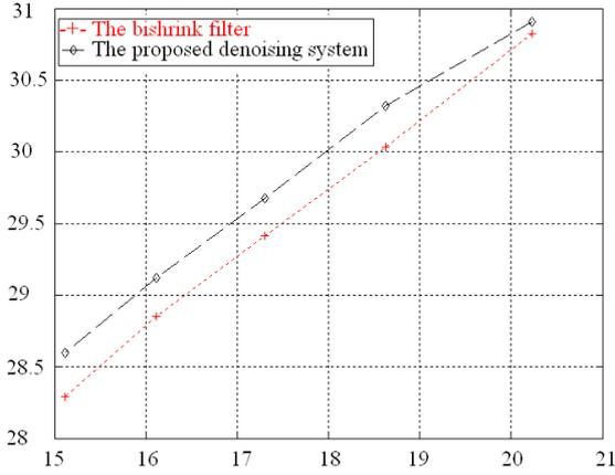
Figure 8. A comparison of the dependencies of the output PSNR on the input PSNR for the bishrink filter and the proposed denoising system for the image Peppers.
