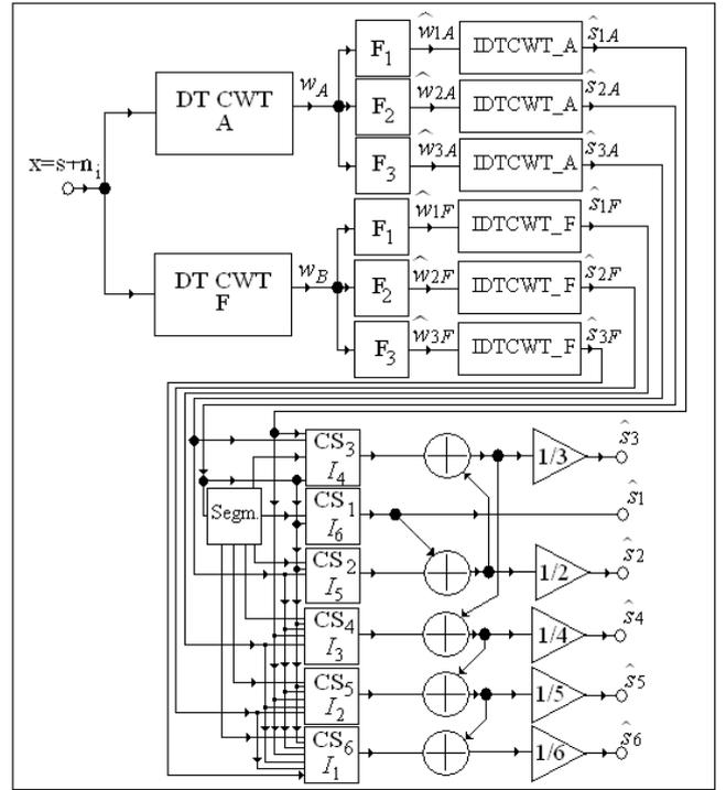
Figure 1. The architecture of the proposed denoising system.
