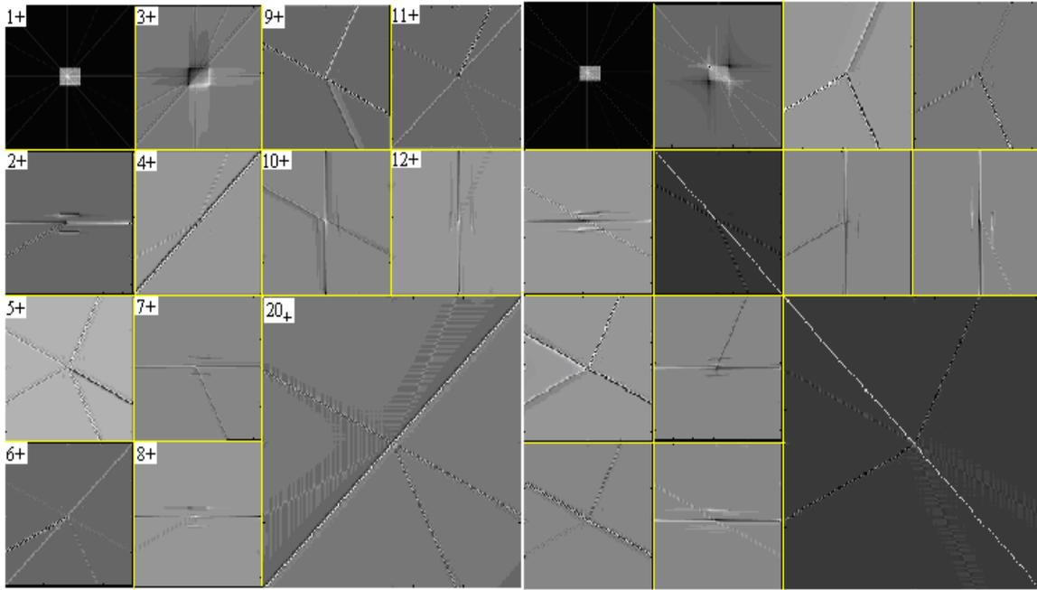
Figure 9. A comparison of two sets of outputs of the HWPT. The outputs corresponding to the coefficients  $\text{Im}\{z_+\}$  are represented in the left picture. The same outputs corresponding to the coefficients  $\text{Im}\{z_-\}$  are represented in the right picture. The left picture contains preponderantly positive angle directions while the right picture contains mostly negative angle directions.
