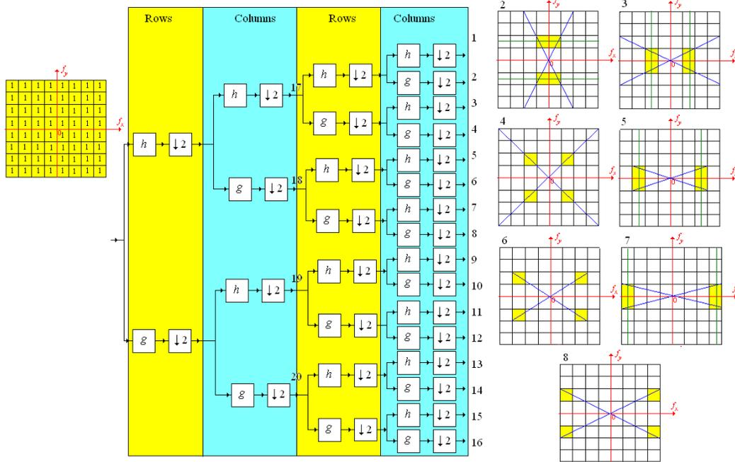
Figure 5. 2D-DWPT with two iterations. The low-pass filter  $h$  and the high-pass filter  $g$  are considered ideal. The images from the first seven detail outputs are marked.
