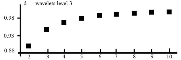
Fig. 2. Degree of shift invariance of HWT as a function of the regularity of the mother wavelet used for its computation.
