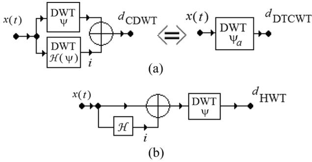
Fig. 1. Implementations of (a) the DTCWT and (b) the HWT are equivalent.
