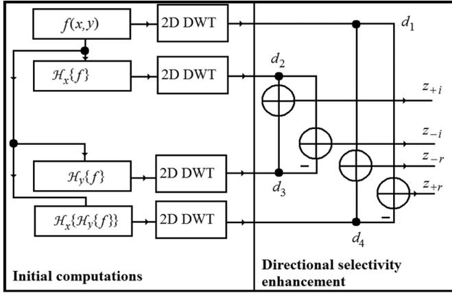
Fig. 3. New 2-D-HWT-implementation architecture.
